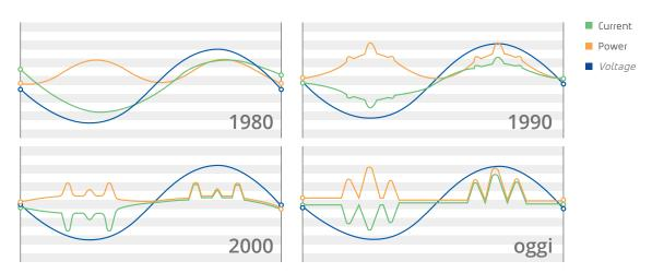
Until the 80's, in all industrial and commercial sites the linear loads were largely prevalent; that is, electrical loads not influenced by power electronics.
